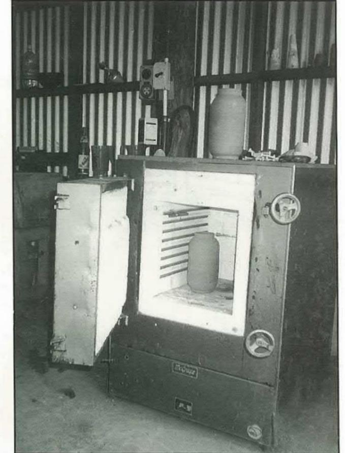
Kiln with thermostat and water gauge
