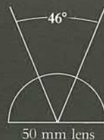
Diagram 4 Angles of view of the three lenses used to take the photographs shown above.
