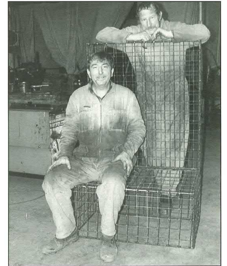
Doug Williams and Murray Rennie make up the steel mesh frame as an armature for the ferro-cement
