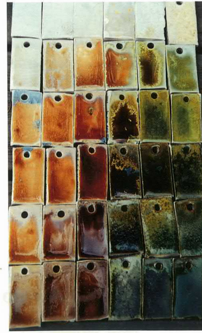
Test tiles by Julie Brooke. Cross blend of Titanium and Nickel to 10%. Crystalline Glaze Base #2, Ceramic Spectrum , page 118.
