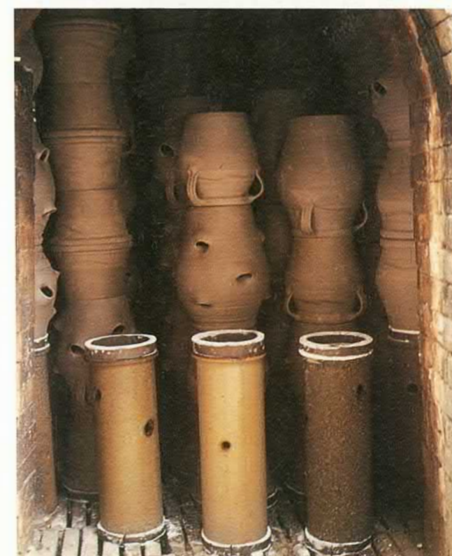
Bardon Mill Pottery. Salt-glaze kiln. Cool spot near door has columns to lift pots for better firing.
