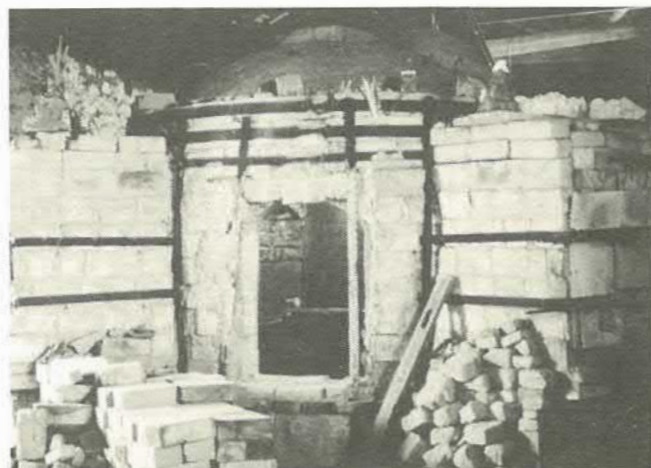
Peter Smith's coal-fired earthenware kiln. Downdraught with fireboxes placed high up.
