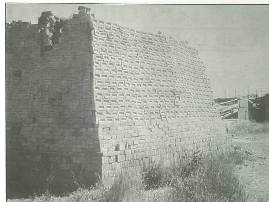
Rear view of the clamp showing fire holes close to the bottom corner
