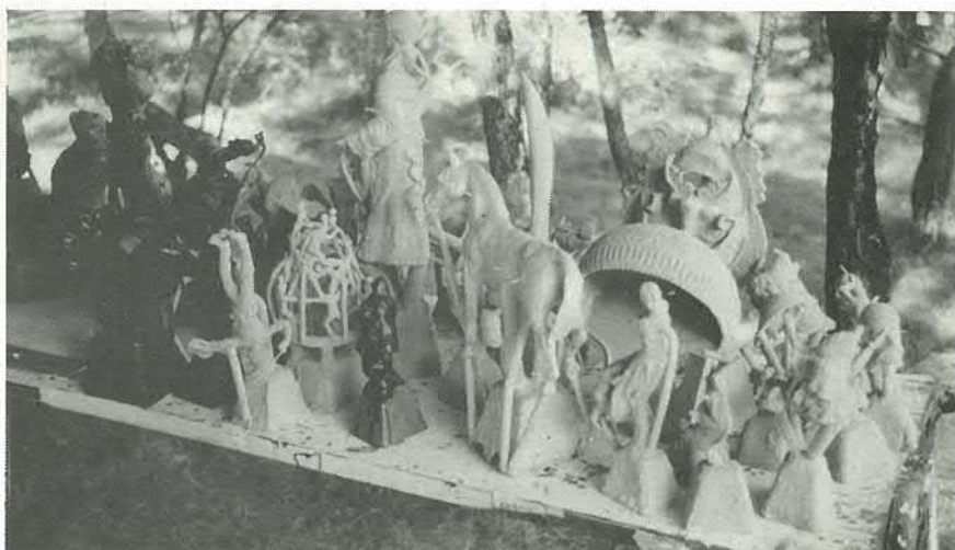
Sprued and cupped waxes, some with first ceramic coat.
