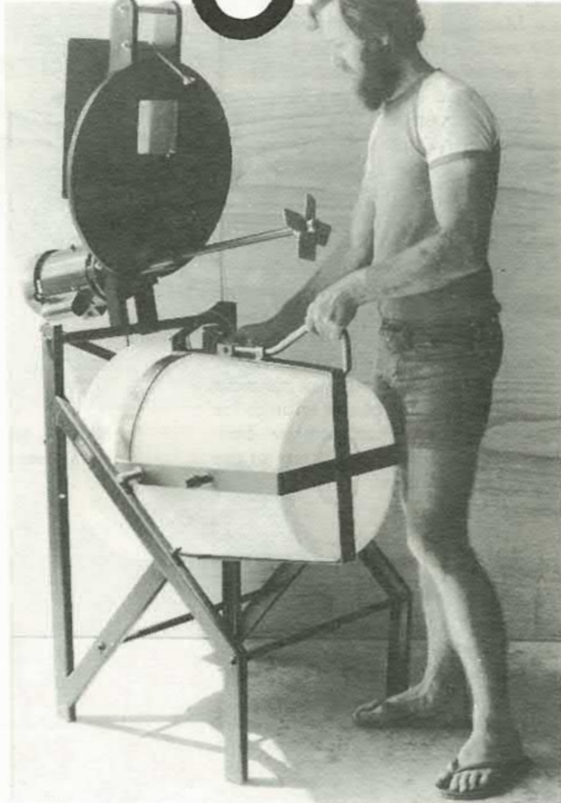
Mixed slip is tipped without heavy lifting. Lifting lid automatically stops motor
