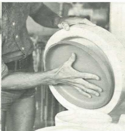
Firm but still pliable cast is removed from mould.
