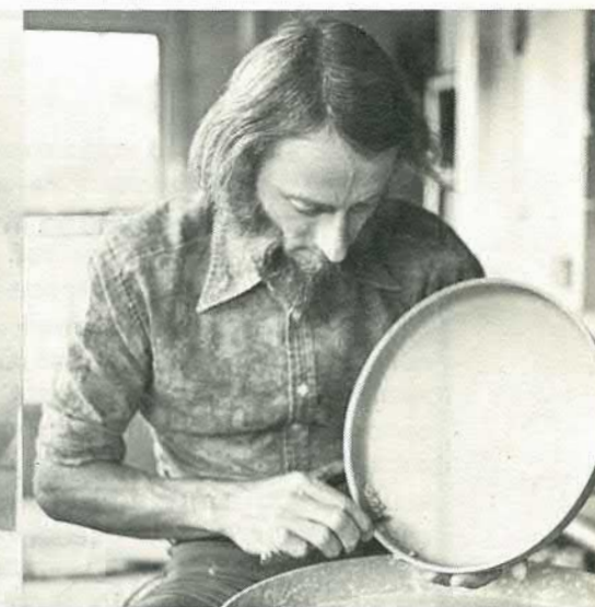
Leather hard cast is fettled with surform blade and knife, then sponged smooth photos: Brian Wilson drawings: Howard Williams
