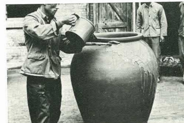
Raw glazing of large jar — Soochow. Normally the pot would stand on a dish to catch run-off.
