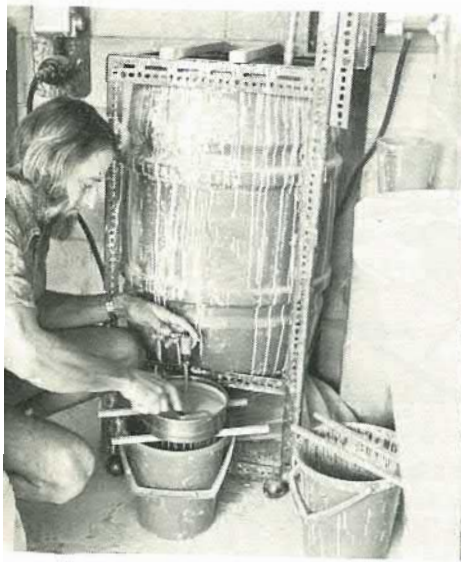
Slip from blunger is screened through 80 mesh sieve before use
