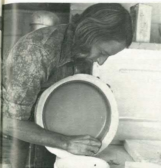
Cast now lost its shine and is beginning to shrink away from mould walls. Spare clay from draining is being trimmed off.
