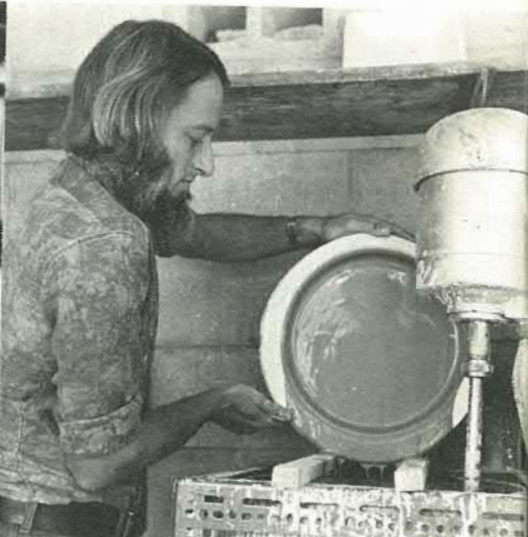
After casting, excess slip is poured back into blunger and mould left to drain.
