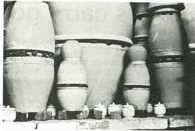
Loaded for the kiln — Yheising. The largest pieces are slab built — the next largest are formed inside a canvas bag.
