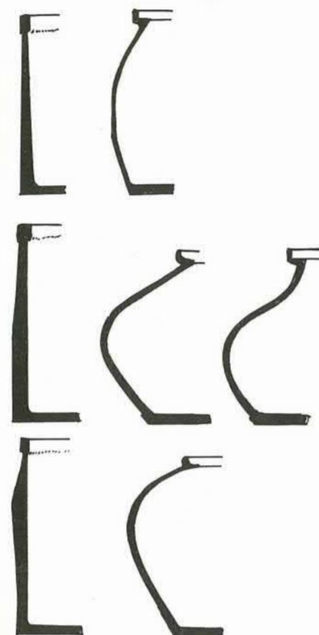
Fig. 5 The relation of shape, pouring angle and lid type.
