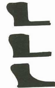
Fig. 1 Base interior radius, correct, too sharp, too slack.
