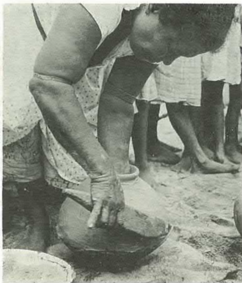
Porobada. Shaping and smoothing with paddle and anvil.
