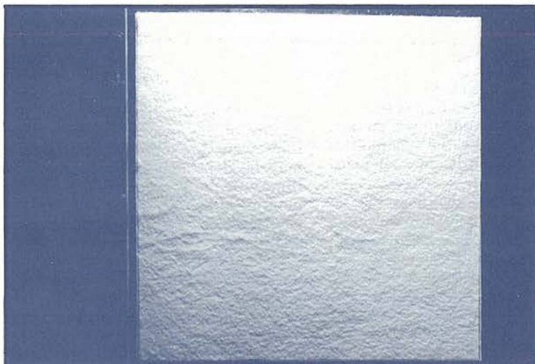
Panel made up — raking light to show texture of filter media.
